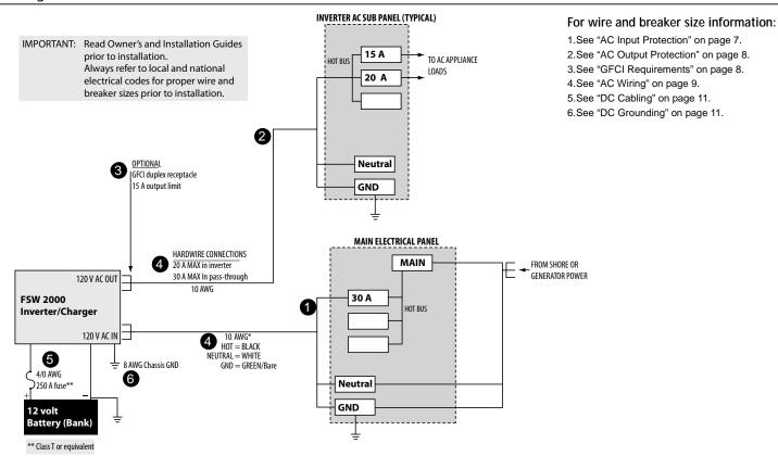
Figure 3 Wiring and Breakers Block Diagram
